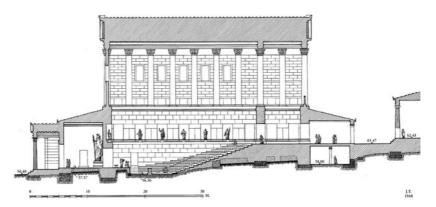
Figure 52. Cross section of the Odeion, 1st phase (late 1st century B.C.), looking east.
