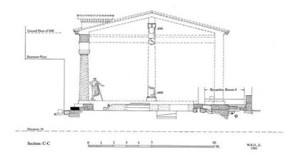
Figure 65. Cross section of the Stoa Poikile, with Doric columns outside, Ionic within; ca. 470–460 B.C.
